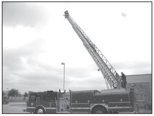
**Above:** The aluminum ladder is hydraulically raised, lowered, rotated 360 degrees, and extended to a full length of 75 feet (a 7-story building).
