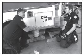
**Stabilize the Load:** Wood blocks are placed under and around the lifting bag to support the raised vehicle, as shown by Brock and Firefighter/EMT Jeff Carey.
