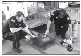
**Lift the Load:** Firefighter/EMT Tyler Hundt lays out pneumatic lifting bags, which are made of aramid-reinforced rubber (left). The largest bag lifts 26.5 tons to a height of 12 inches. Paramedic Richard Brock (right) operates a control that inflates a lifting bag with air.
